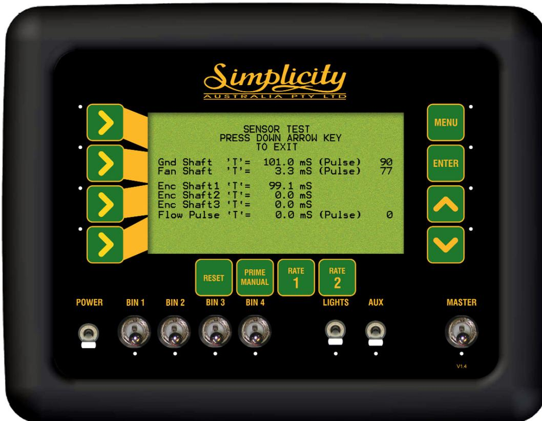
Sensor Test Screen (Hydraulic)
