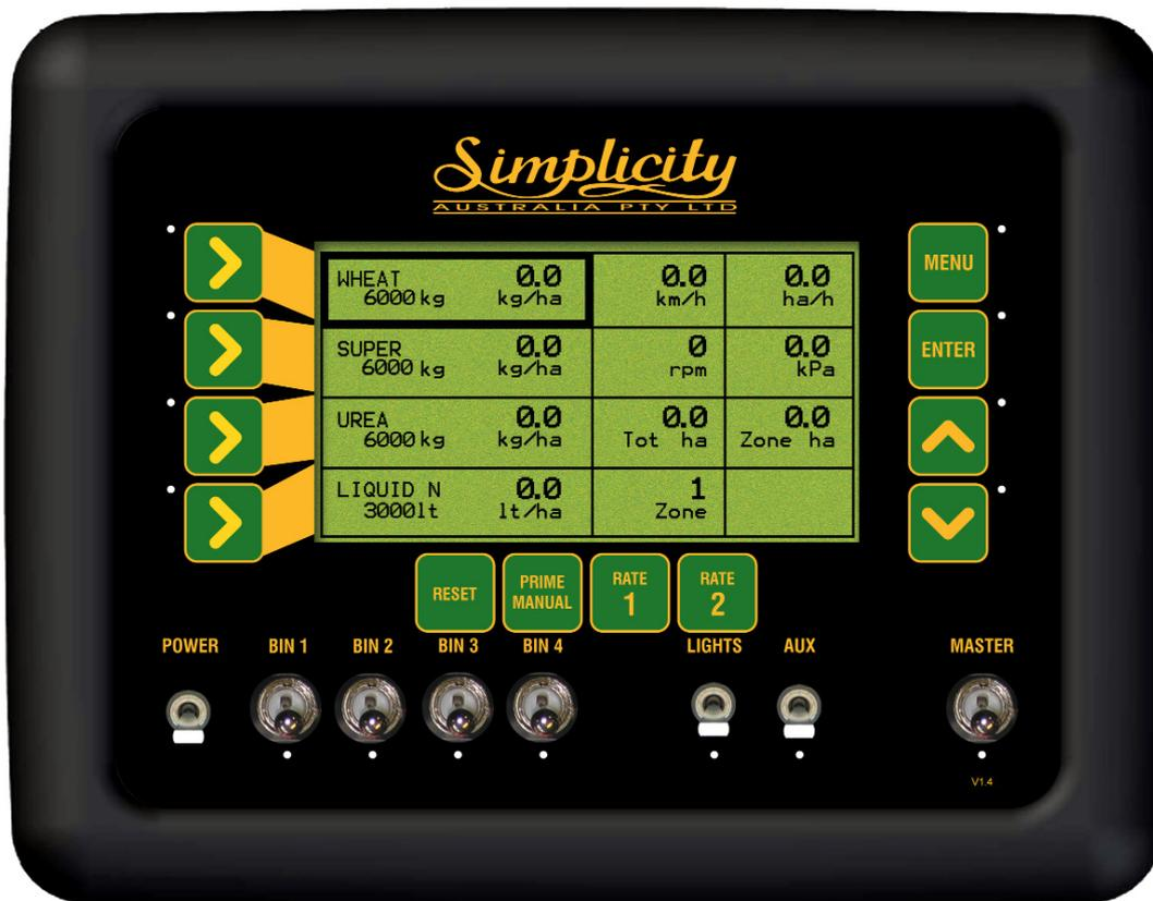
Working Screen with a Liquid Tank
