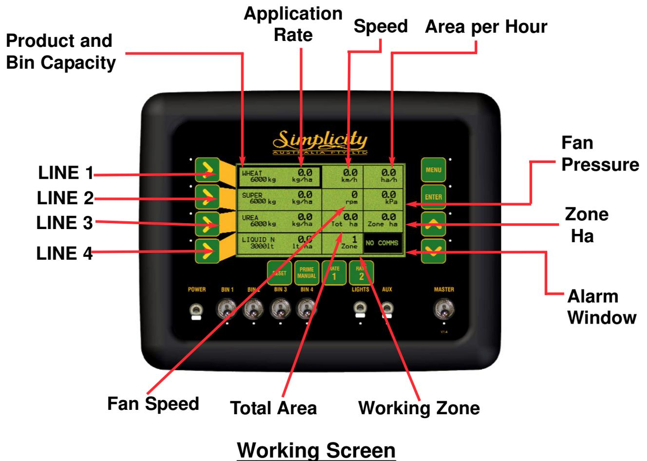
**PRODUCT AND BIN CAPACITY-** Shows the four bins down the left hand side of the console, starting with Bin 1 at the top through to Bin 4 down the bottom. If only two bins are selected from the SEEDER SETUP MENU then LINE 3 AND LINE 4 rows will be blank.
