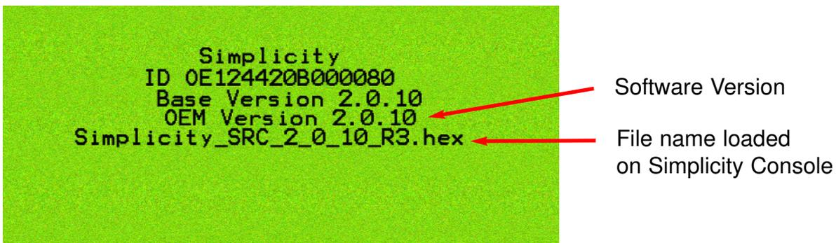
The above screen is displayed for 60 seconds each time the Simplicity Console is switched ON, using the 'POWER', button.
